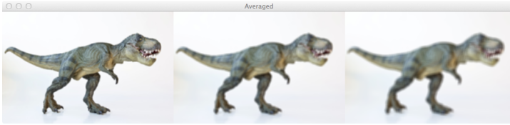
Figure 8.2: Performing averaging blurring with a 3 \times 3 kernel ( left ), 5 \times 5 kernel ( middle ), and 7 \times 7 kernel ( right ).
