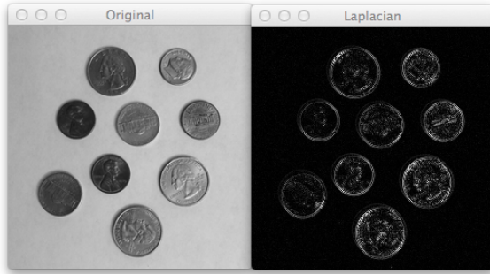
Figure 10.1: Left: The original coins image. Right: Applying the Laplacian method to obtain the gradient of the image.
