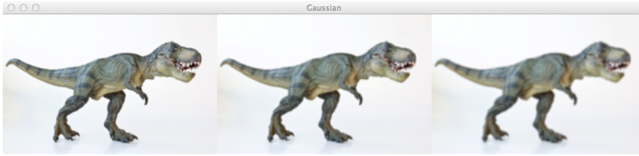
Figure 8.3: Performing Gaussian blurring with a 3 \times 3 kernel ( left ), 5 \times 5 kernel ( middle ), and 7 \times 7 kernel ( right ). Again, our image becomes more blurred as the kernel size increases, but is less blurred than the average method in Figure 8.2.
