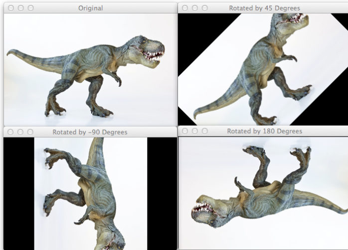
Figure 6.2: Top-Left : Our original T-Rex image. Top-Right : Rotating the image by 45 degrees. Bottom-Left : Rotating the image by -90 degrees. Bottom-Right : Flipping T-Rex upside down by rotating the image by 180 degrees.
