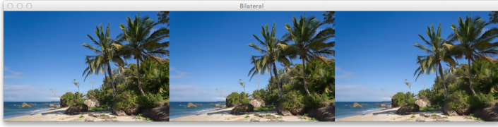
Figure 8.5: Applying Bilateral blurring to our beach image. As the diameter of the neighborhood, color \sigma , and space \sigma increases (from left to right), our image has noise removed, yet still retains edges and does not appear to be “motion blurred”.
