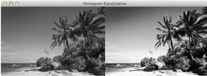
Figure 7.4: Left : The original beach image. Right : The beach image after applying histogram equalization.
